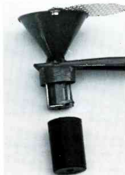
FIG. 4—A 35mm FILM CANISTER provides a water-tight enclosure for the solenoid valve.
